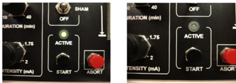
Figure 10: Different stimulation conditions: active vs. sham. Some tDCS devices provide set ups for active and sham condition. Usually applicable stimulation is indicated with a light signal.
