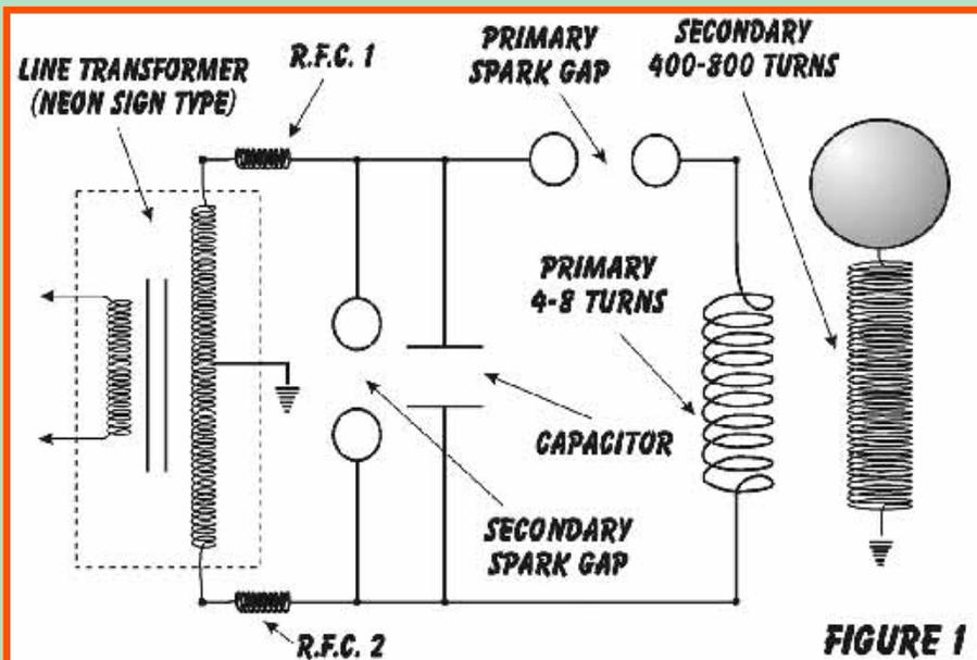
needed to supply enough energy to the capacitor so that it can “kick” out pulses at a very high speed (600 kHz is common) and not be depleted. The idea is that as a charge builds up in your capacitor, it eventually becomes large enough to arc across the spark gap.
